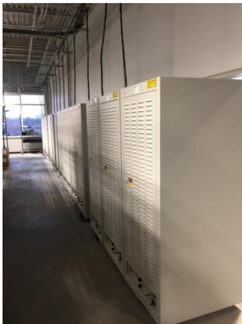
Figure 2 - NHR 9200 Battery Test Systems (back side of test equipment) at A123 Systems R&D Laboratory
